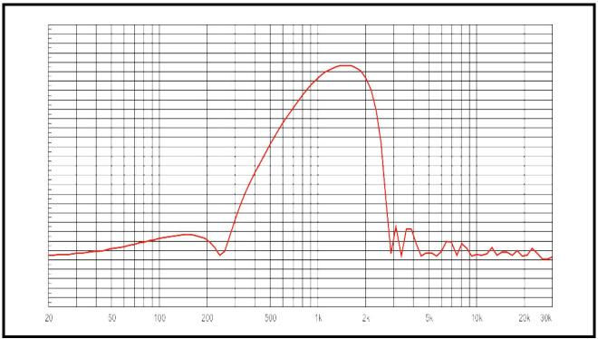
FIGURE 28. Frequency Response - Preset 3 (900Hz to 2100Hz)
